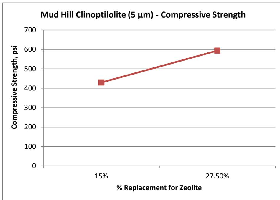
Figure 1: Compressive strength for 5µm Mud Hill Clinoptilolite using Class H cement
