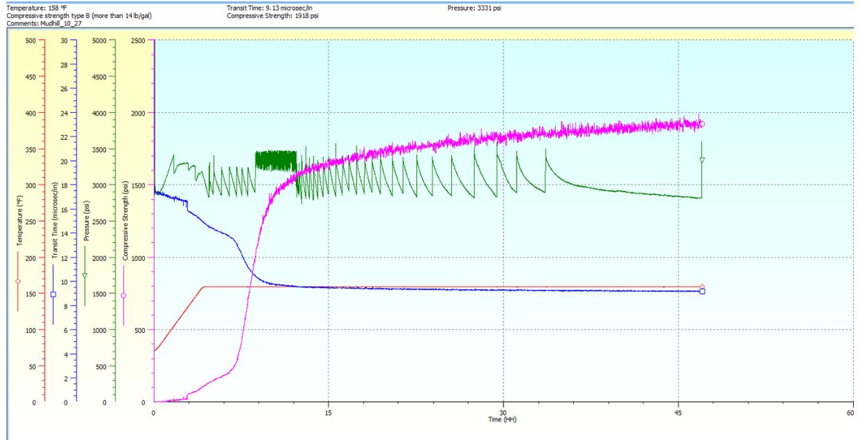
Figure 2. UCA analysis of 10 $\mu$ m mudhill at 27.5% replacement level at 70°C. The pink/purple curve is the compressive strength and correlates to the first y-axis (far right).
