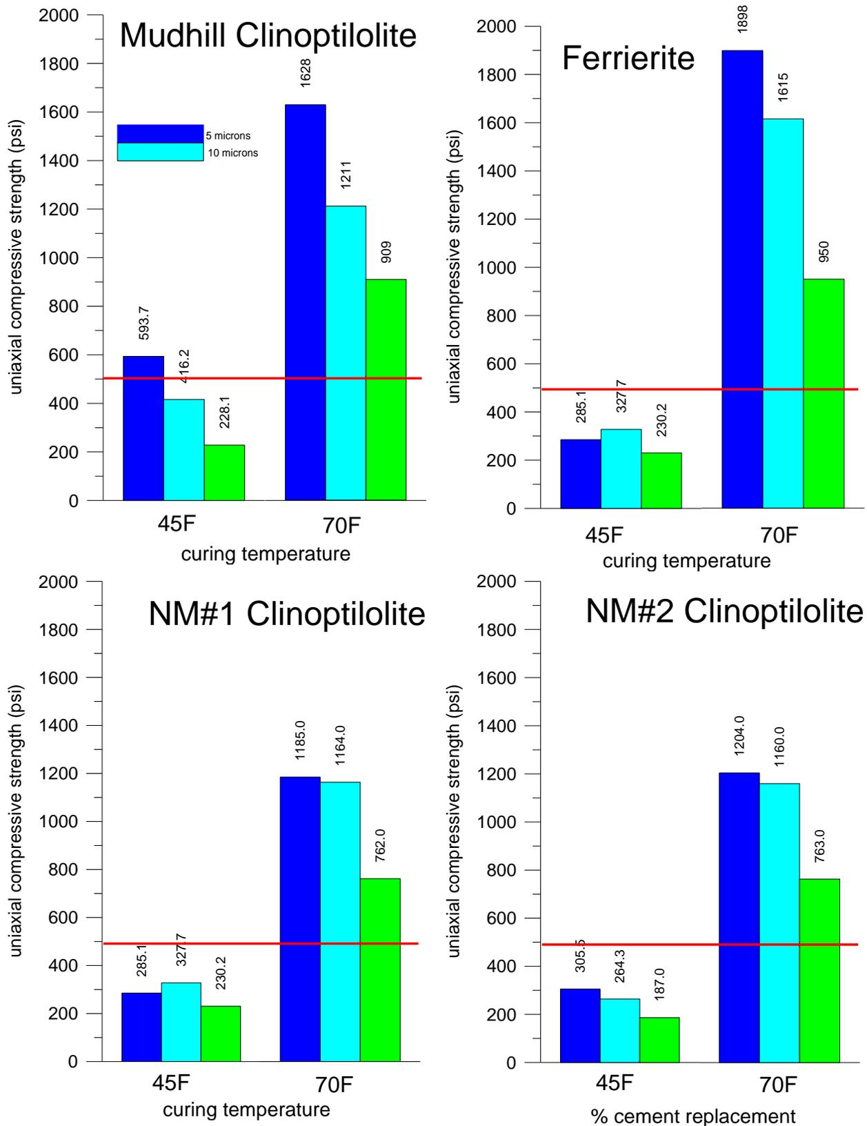
Figure 1. The 24 hour compressive strength is provided by mudhill, ferrierite, NM#1, and NM#2 as a function of curing temperature.
