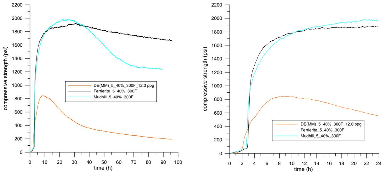
Figure 2. Real time compressive strength development for the 40% replacement level using 5 micron ferrierite, mudhill clinoptilolite, and diatomaceous earth (MM) at 300°F and 5000 psi.
