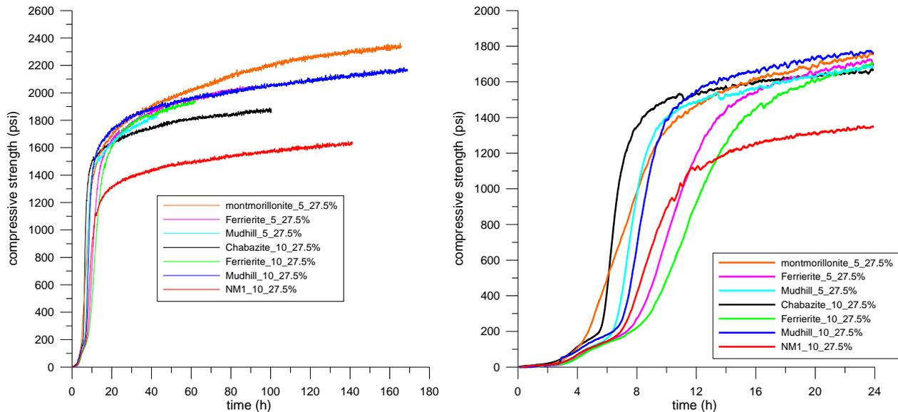
Figure 1. Real time compressive strength test at 27.5% replacement levels. Test conditions: 70°C, pressure ~3000 psi.
