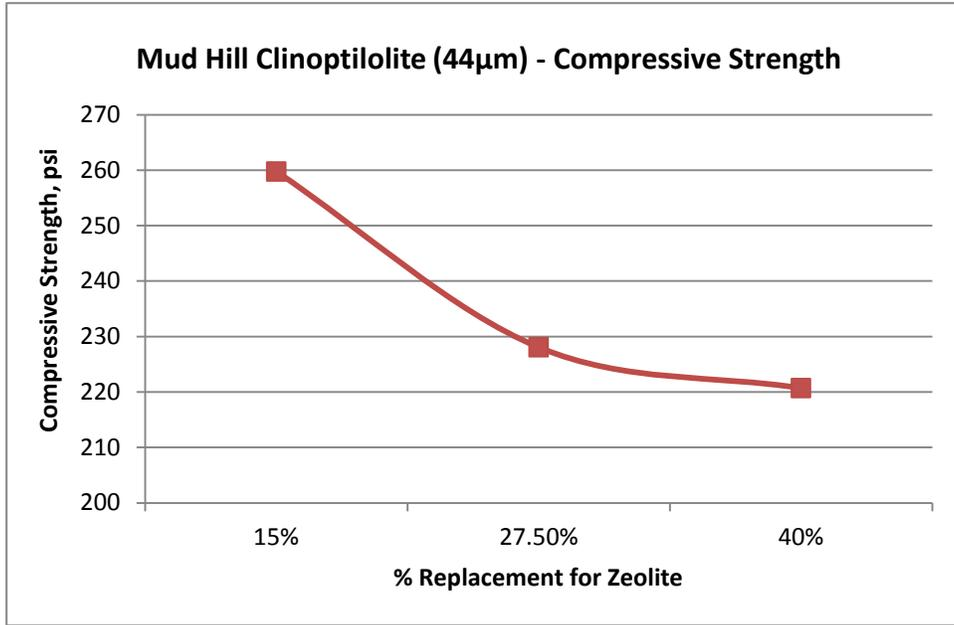
Figure 1: Compressive strength for 44µm Mud Hill Clinoptilolite using Class H cement
