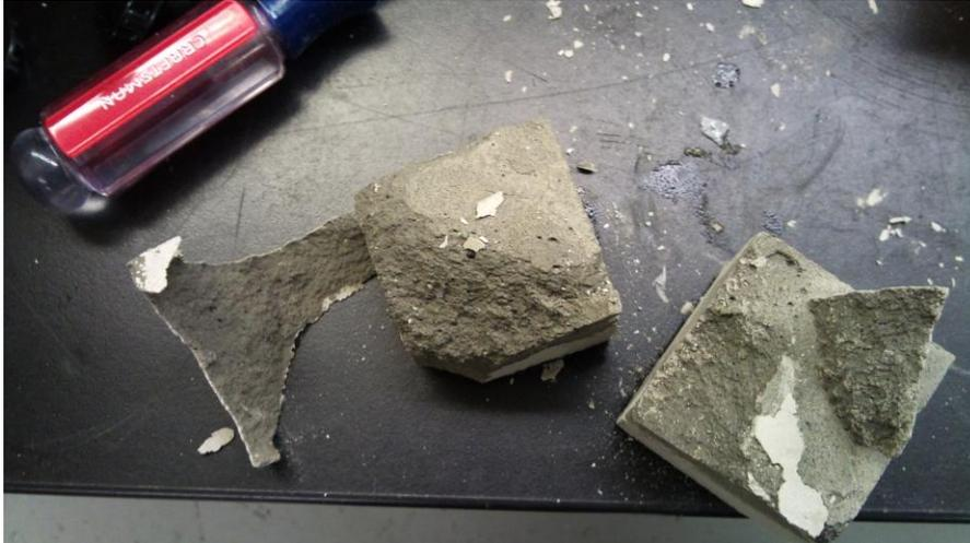
Figure 1 Damaged Ferrierite samples while de-molding
