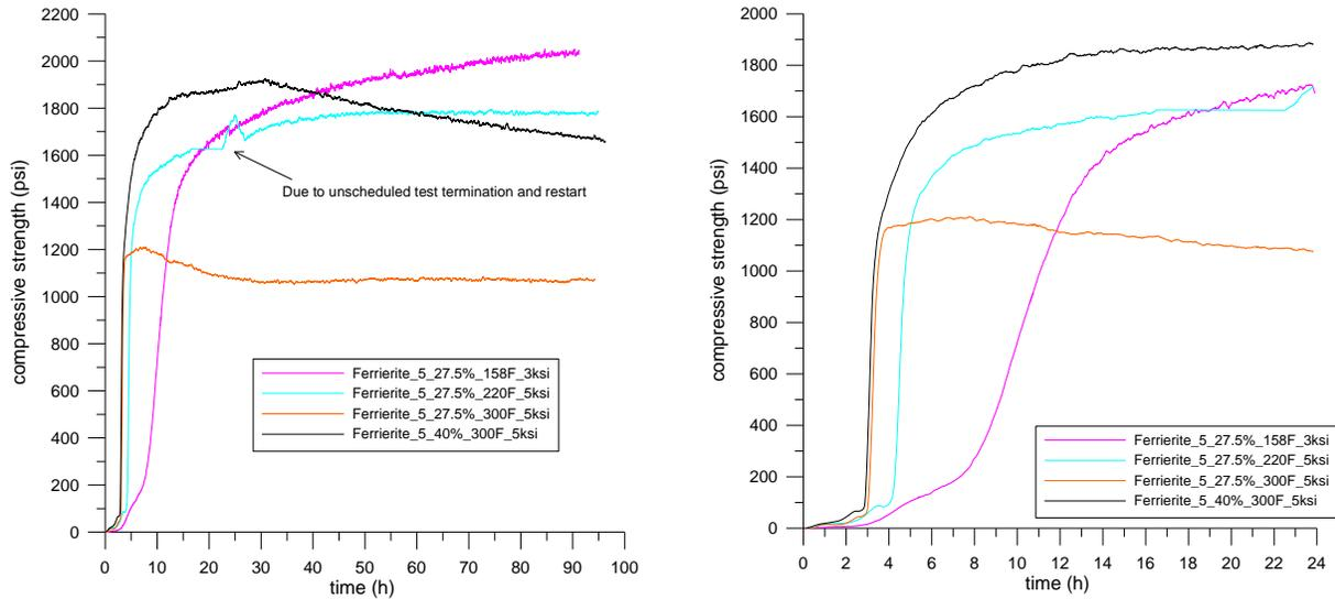
Figure 1. Real time compressive strength development for ferrierite (5 micron) based cement mixes at temperatures ranging from 158°F to 300°F. Target density 13.5 ppg.
