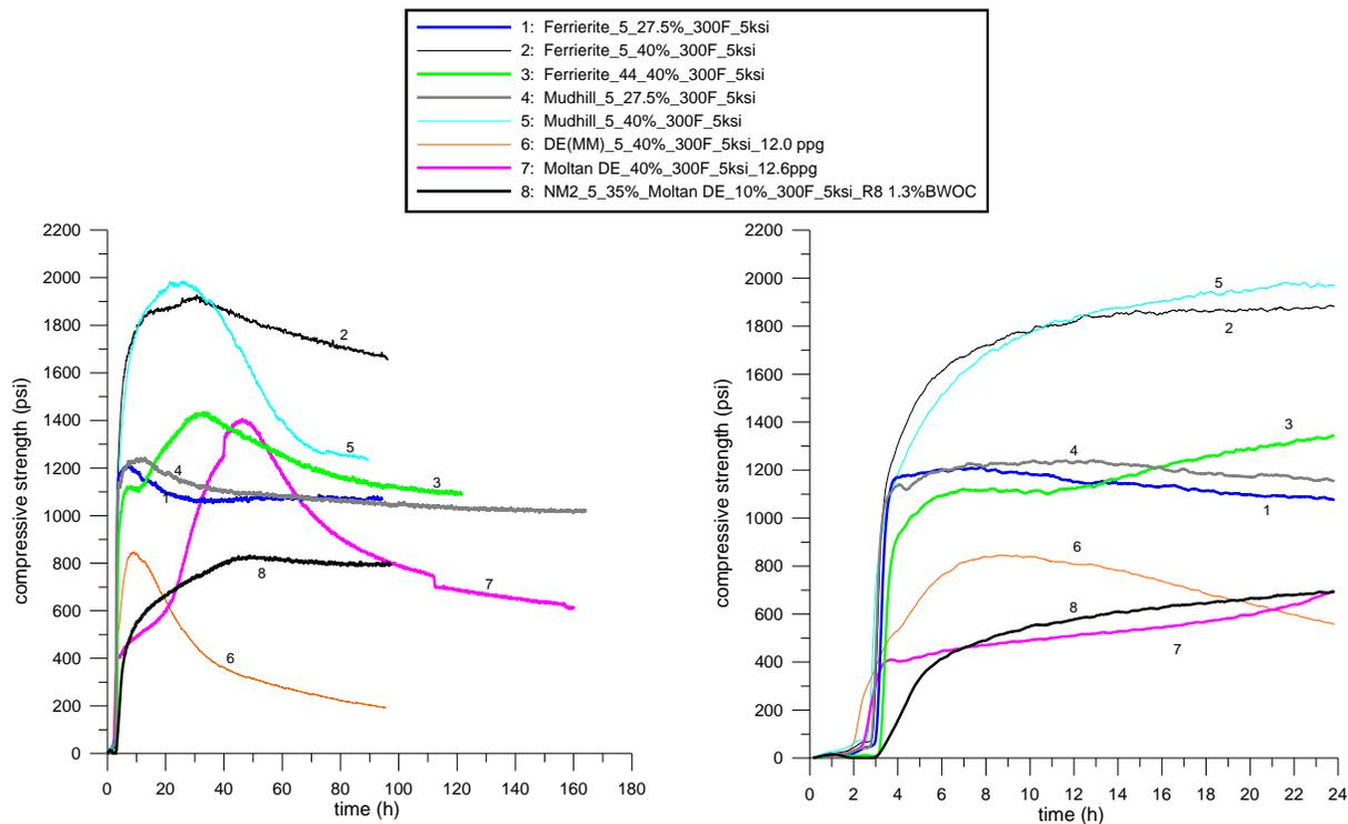
Figure 3. HPHT UCA test results for tests conducted at 300°F and 5000 psi.
