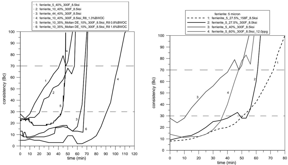
Figure 1. Consistency plots for ferrierite based mixtures. Temperature ramping schedules: 300°F (60 min).
