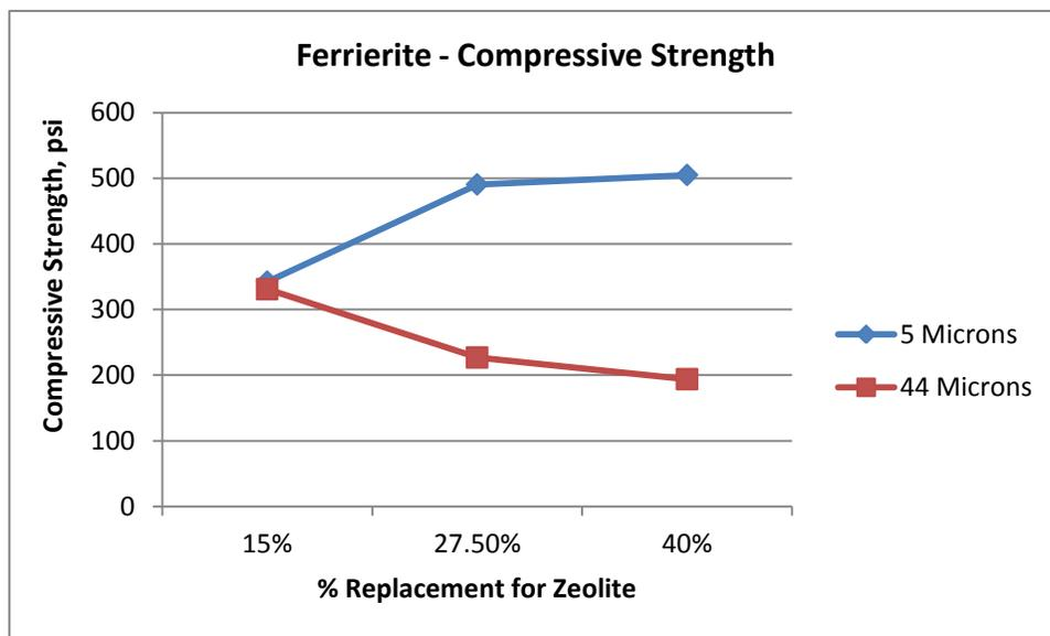
Figure 2 Compressive strength results for Ferrierite.
